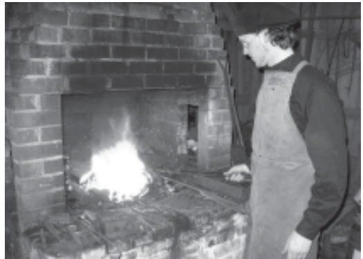
Blacksmith Joe Moquin (below) prepares to use hand forged tongs to pull heated metal from the fire.
